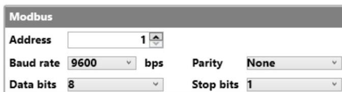
The image shows a 'Modbus' configuration window with the following settings:
