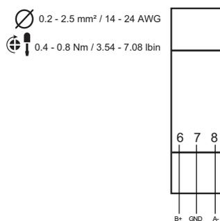
**Fig. 8** Porta RS485
