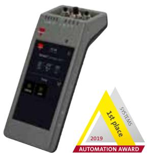
After plugging in the sensor to one of the integrated M12 or M8 connectors, it will automatically download the IODD file, through Wi-Fi and display all data immediately. Through a 5.5" HD touchscreen display and user-friendly interface the user can view, modify, and optimize even the most complex device very quickly.
